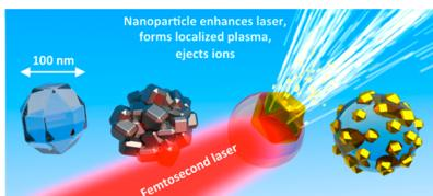
In a new study, Hickstein *et al.* (DOI: 10.1021/nn503199v) overcome these hurdles through a new method that images localized nanoscale plasma created when an isolated nanoparticle is irradiated with a short but strong laser pulse that is slightly below the plasma formation threshold of the bulk material. Here, the nanoparticle itself enhances the laser field in localized regions, ejecting ions in a direction that can be used to determine
