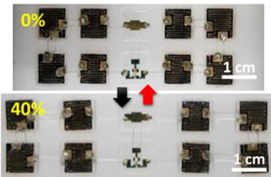
with a high Young's modulus, while the thin film is made of a mixture of Ecoflex and PDMS with a significantly lower Young's modulus. On the stiff islands, the researchers placed microsupercapacitors composed with layer-by-layer assembly of multiwall carbon nanotubes with metal oxide and polymer electrodes.
